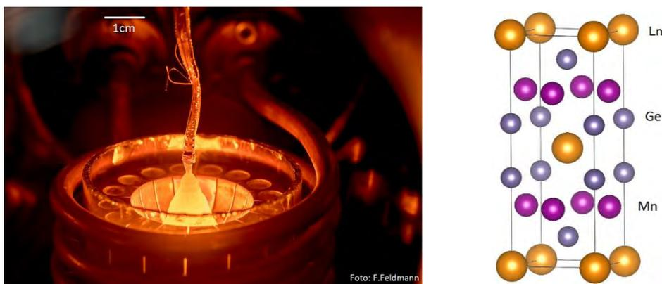
Fig. 1: *Left*: Crystal growth by Czochralski method from a levitating melt. *Right*: ThCr<sub>2</sub>Si<sub>2</sub>-type structure of the LnMn<sub>2</sub>Ge<sub>2</sub> compounds.
