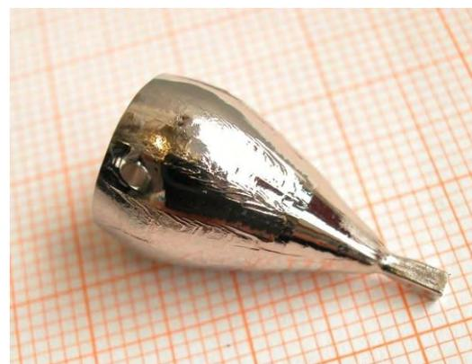
Fig. 2: Ga<sub>0.8</sub>Ge<sub>0.2</sub>Pd<sub>2</sub> single crystal, grown with the Czochralski technique in [001] direction.
