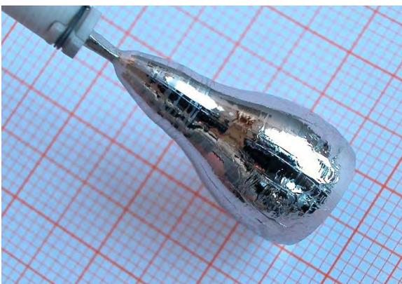
Fig. 1: Ga<sub>0.7</sub>Sn<sub>0.3</sub>Pd<sub>2</sub> single crystal, grown with the Czochralski technique in [010] direction.
